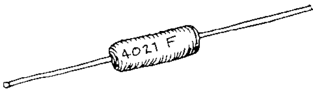
metal film 1% precision resistor
